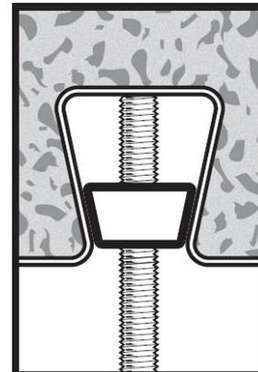
Rotate the threaded rod in to the Wedge Nut so that the rod touches the top of the rib (Finger tight). Check the tapered faces of the Wedge Nut touch the faces of the rib profile.
