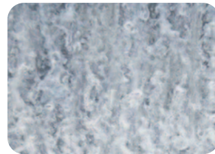
Zinc-magnesium Coating Thickness: 7 \mu\text{m}
